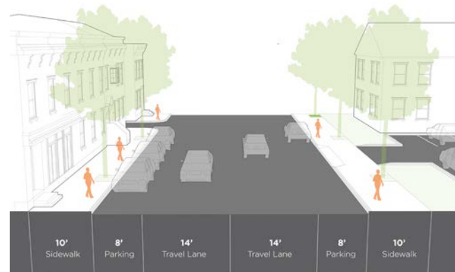
EXISTING SECTION LOOKING SOUTH ON FRONT ST.
